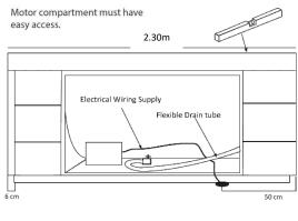
**IMPORTANT:** Important: The equipment must be connected to an exclusive and permanent power line capable to support installed power. Lighting and electrical receptacles must be located at least 1.5 meters from the equipment.
